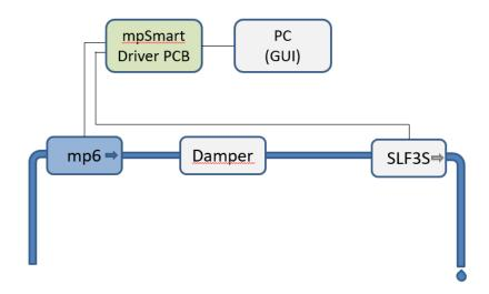
For the wiring, use the included cable to connect the mp6 and SLF3S-1300F to the Flow Controller and the USB cable to connect the kit with your PC / Laptop.
