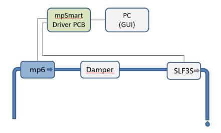
For the wiring, use the included cable to connect the mp6 micropump and SLF3s-0600F to the Flow Controller and the USB cable to connect the kit with your PC / Laptop.
